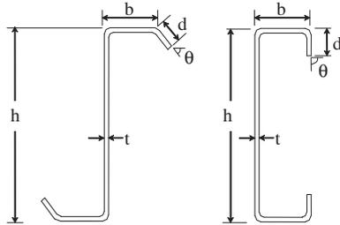
Fig. 3. Definitions for dimensions of Z and C sections.
