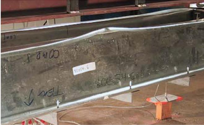
Fig. 2. Distortional buckling modes of a cold-formed steel C section in bending [2].
