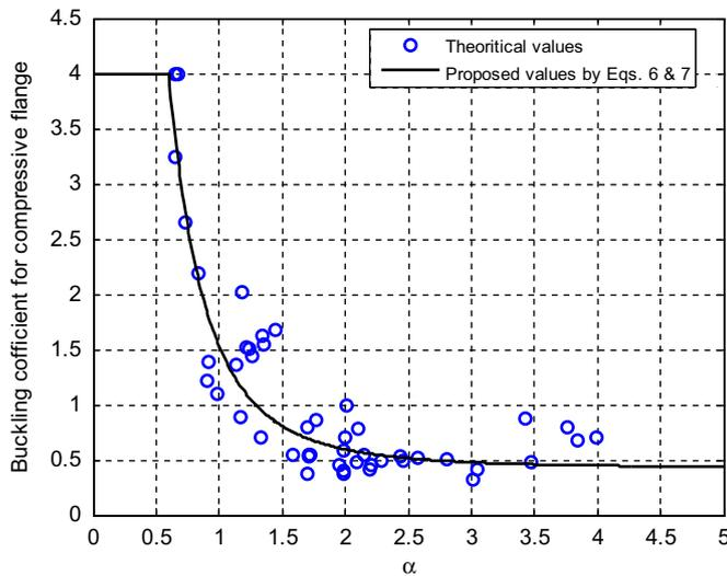
Fig. 4. Comparison of the proposed equations with the theoretical values.
