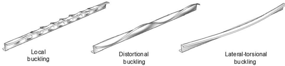
Fig. 1. Buckling modes of a cold-formed steel Z section in bending.
