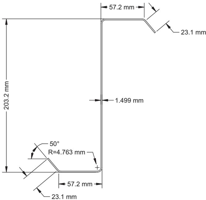
**Fig. 5.** Cross-section of 8ZS2.25 × 059.
